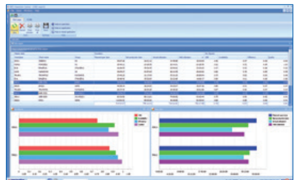
Example of an OEE index and its elements displayed in the MES system HYDRA.
